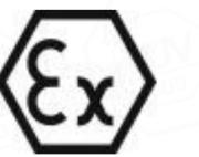
II 1/2G Ex db h IIA T3 Ga/Gb (motor + pump) **II G IIA (flame arrestor)**
