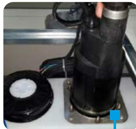
**REINFORCED BRACKET FOR SUBMERSIBLE PUMP ASSEMBLY**
